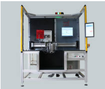
Safety test system for pump motors
